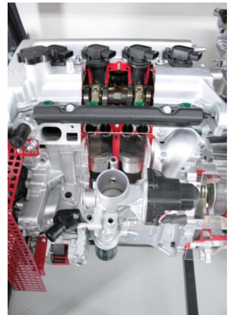
Image shows the sectional view of the 4 cylinder combustion engine
