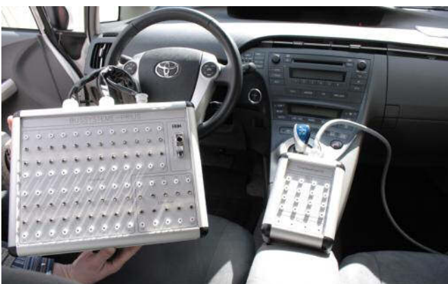
Image shows on the left the measuring box with CAN- and LIN-BUS interfaces and on the right for the door control unit
