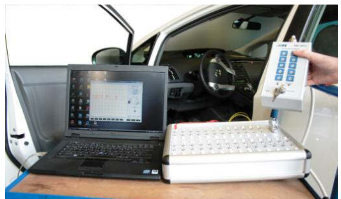
Image shows the direct measuring of the CAN-BUS signal with the PC-memory-oscilloscope and the possibility of the fault switch
