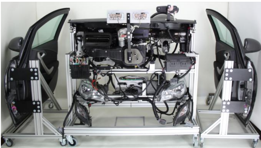
Image shows the training stand instrument panel CAN- / LIN-Bus with original instrument panel, driver and front passenger airbag, the complete lighting system and the instrument lighting of an Astra J.
