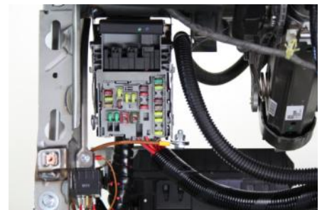
Image shows the fuse box
