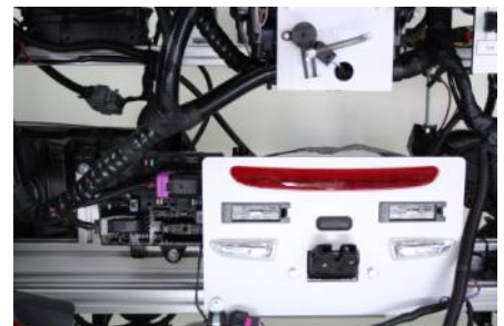
Image shows board with tailgate elements and side turn signals as well as the rear electronics module
