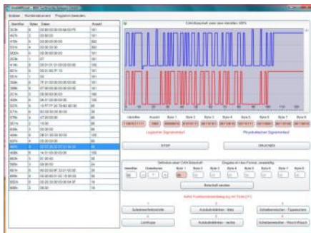
Illustration shows the overview of the CAN-BUS messages and presentation of a selected message as oscilloscope illustration.
