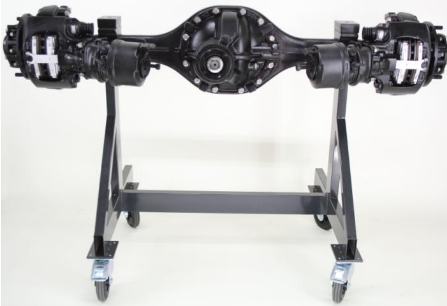
Image shows the front view of the rear axle with disc brake Order-number 0090 1520
