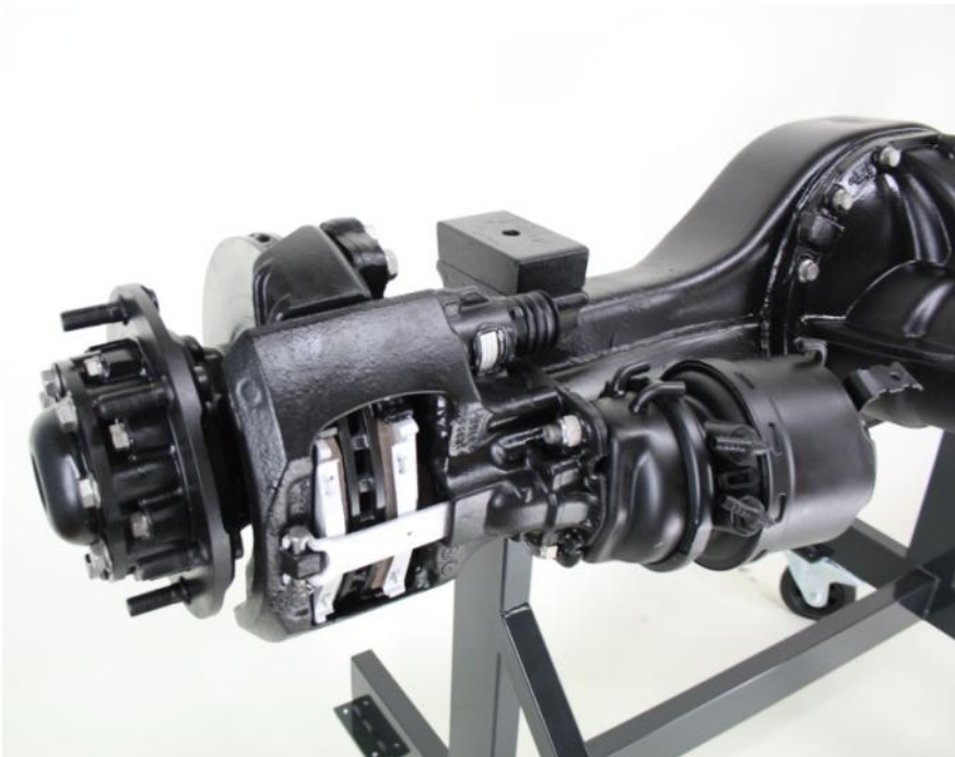
Image shows a detail view of the rear axle with disc brake
