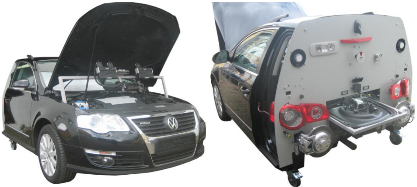
Image shows Vehicle functional model VW Passat Blue TDI Order-number 0000 9358 with additionally applied error circuit for the engine management and the CAN-BUS system, as well as integrated test adapter.
