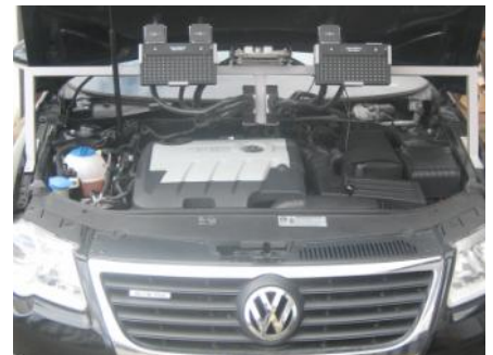
The illustration shows the engine room with attached interfaces and test kits for garage-oriented measuring.
