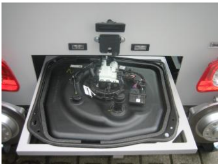
The image shows the heated auxiliary tank (17 l) for the urea solution (AdBlue), which is integrated in the spare tire well of the vehicle.
