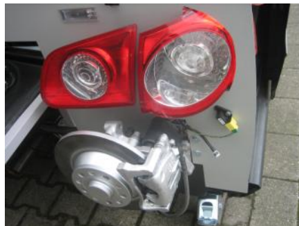
The illustration shows the functional electrical parking brake.
