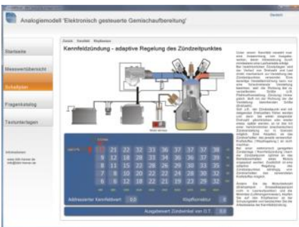
Operating procedure of a mapped ignition with adaptive knock control. Two-dimensional map, addressed by engine speed and load. Characteristic values can be edited as desired.
