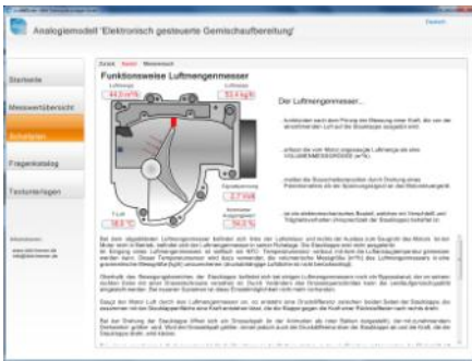
Air volume meter, animated presentation, explanation of the function mode. Computation of air mass from the air temperature (influence of the induction air temperature).
