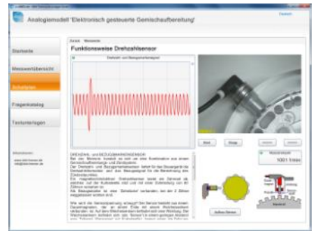
Speed and reference mark sensor. Explanation of the function mode, oscilloscope presentation of the sensor signal depending on the engine speed.
