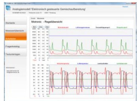
Graphical representation of the engine operating parameters as continuous lines printout.
