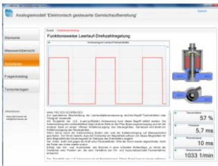
Idle adjustment. Explanation of the function mode, oscilloscope presentation of the adjustment activation depending on the desired engine number of revolutions which can be regulated.
