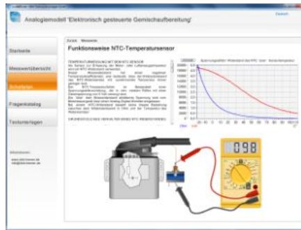
NTC sensor cooling-fluid. Explanation of the function mode, mounting of a sensor characteristic, notes for the fault diagnosis.
