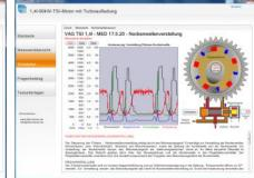
Explanation of variable valve timing with the original signal image of the sensor signal and the injector actuation.
