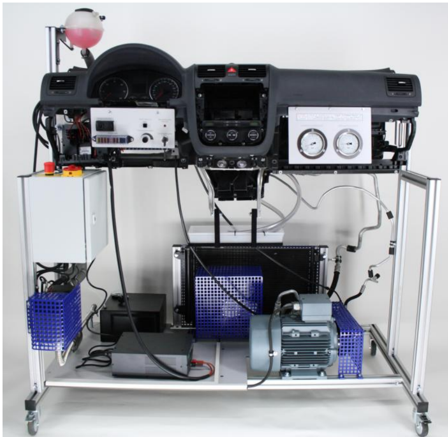
Image shows the training stand VW-Climatronic with auxiliary heater Order-number 0000 2635
